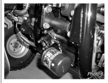
Oil Cooler Plumbing: proper hose installation Continue through the following steps if you are now using the installed Jagg 4800 oil filter adapter to feed oil to a Jagg oil cooler and return it to the engine.
