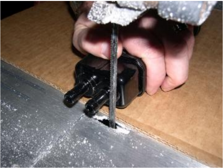
Photo 1. Cut off nipple flush to boss.
