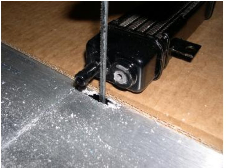
Photo 2. Cut off nipple flush to boss.
