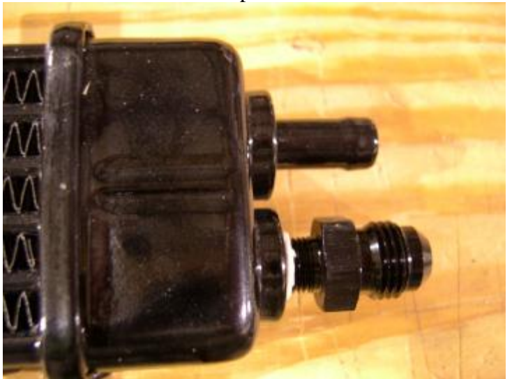
Photo 12. Illustration of made port 1/8" - AN6.
