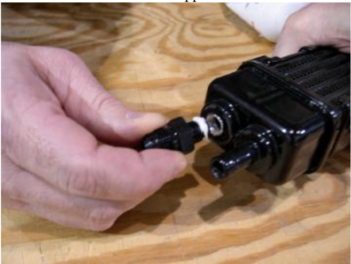
Photo 9. Install doped fitting to finger tight.
