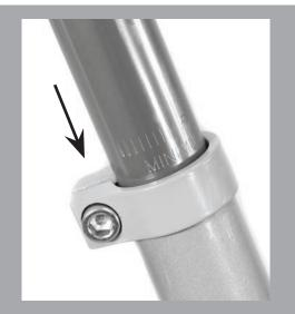
The seat post "minimum insertion/maxiumum height" marking should **NOT** be visible when the seat post is inserted into the seat tube.
