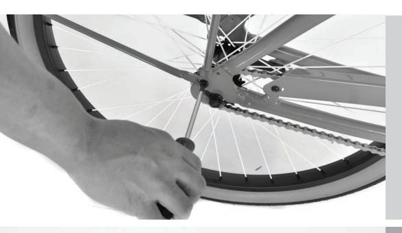
Align the rear fender brace hole to the correspond next to the rear wheel hub and screw into place.
