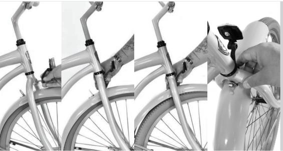
With fender tab on the back of the fork, slide the long screw through front fork hole and fender tab, with a washer on either side of the fork. Screw into place.
