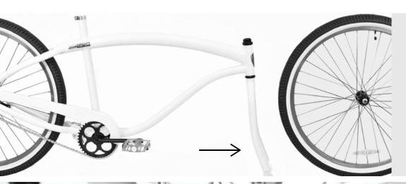
Locate the front wheel. Hold the bike in an upright position and lift the front fork of the bike upwards. Make sure the curve of your fork is oriented in the correct direction. (see reference photo)
