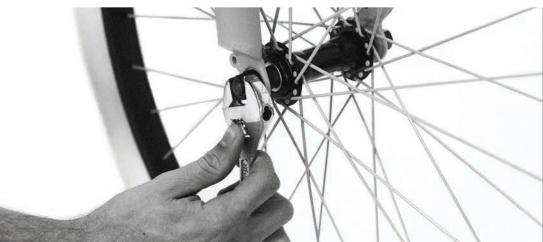
Center the fork onto the wheel. Use the 15mm wrench to turn the right axle bolt clockwise until tight. Repeat this step on the left axle bolt.
