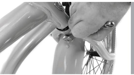
Check the fender and make sure it is centered over the tire. If the fender is not centered, you can adjust the fender braces by hand. Once it is centered, fully tighten the screws using the adjustable wrench provided (avoid using a screwdriver for this step to prevent stripping the screws).
