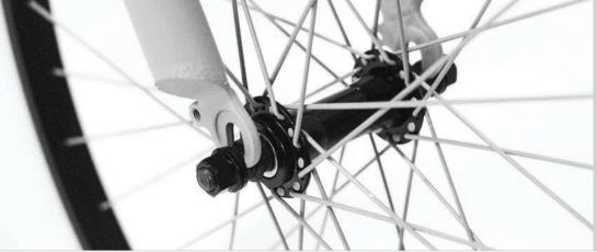
Line up the front fork to either side of the wheel axle and lower the front fork down ensuring that the wheel axle is firmly held in place.
