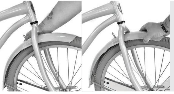
Locate the clear bag labeled "front fender hardware". Inside the bag is a long screw, washers and nut. Carefully slide the front fender through the front fork. Line up fender tab with the hole in the fork.
