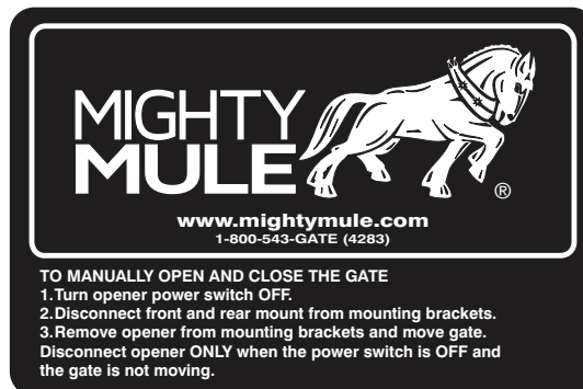
Logo and Manual Disconnect label installed on control box
