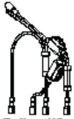
Battery Wire Harness (1) with 15A Access (2)
