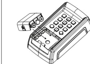
4 REMPLACER CARTOUCHE DE COUVERCLE DE BATTERIE ET FIXER LA VIS.
