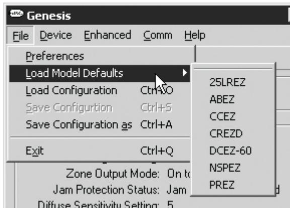
When you select a conveyor model a default configuration for the conveyor model is loaded. In preferences, if the “If device is attached when opening files” is set to “Prompt” the following dialog appears:
