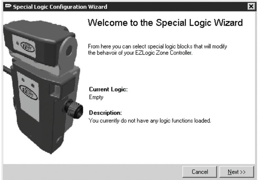
If there is a special logic function already loaded into the zone controller, the name and description of the function will be displayed on this screen. To select the function you wish to load, click “Next”. The following screen appears:
