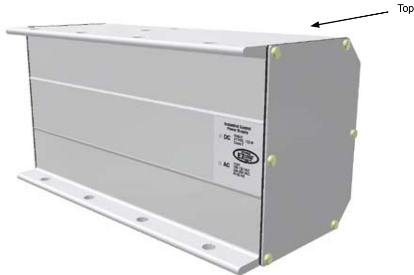
Figure 16—IOP Unit Mounting Position
