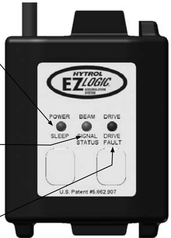
Figure 20—Indicator LEDs—Right Button Pressed
