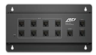
The CB-8 is an installation accessory designed to provide convenient and reliable power connections for up to eight (8) RTI in-wall keypads\*, touchpanels and other devices. In addition to providing power, the CB-8 combines and routes the infrared outputs from the touchpanels to a single output for connection to an RTI control processor. Multiple CB-8 units can be daisy-chained for connecting more than eight devices. A 12VDC 4.0Amp power supply is included.
