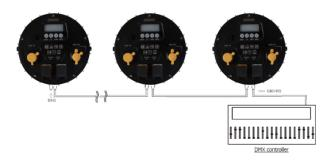
Connect the DMX-output of the first fixture in the DMX-chain with the DMX-input of the next fixture. Always connect one output with the input of the next fixture until all fixtures are connected. Up to 32 fixtures can be connected.
