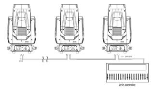
Connect the DMX-output of the first fixture in the DMX-chain with the DMX-input of the next fixture. Always connect one output with the input of the next fixture until all fixtures are connected.
