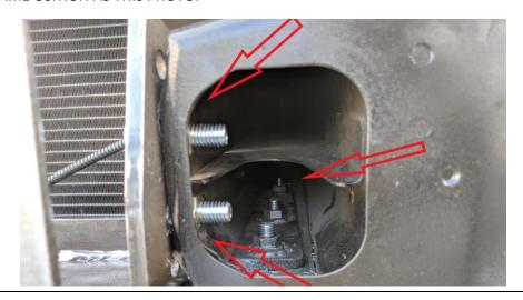
Step 9: Using a table vise, bend the stock hood latch brackets as shown in photo. If you do not have a table vise you may improvise by using the DRAIN holes on the winch plate.
