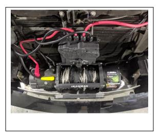
Once mounting and wiring winch is complete, re-install the front bumper. When reinstalling the front grill, you will use two long zip ties to keep the grill in place near the bottom of the grill. The zip ties will wrap around the hood latch brackets and out through the front grill. See photos for example.
