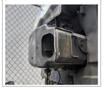
Step 8: a) Insert frame rail sandwich plates into frame rail. B) Mount up winch plate with only four bolts from bottom of plate, two bolts on each frame rail and bolt tight so plate sits flats up against the jeeps unibody. C) Mark the two holes on the side frame bracket which we call "bunny ears". Mark the furthest hole to be drilled under the jeep past the radiator core support. See photos below.
