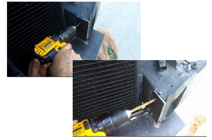
Step 6: Once all 4 holes have been drilled, install hardware, do not tighten.
