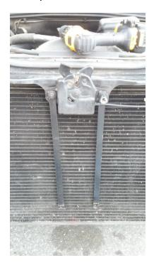
Step 3: Be sure bracket is installed behind latch release cable.
