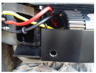
This is where we mounted our solenoid and this is all covered by the bumper. The two black plastic pieces you see to the left of the winch, is what's inside the big black box that goes on top of the winch. Every winch has a different looking solenoid.
