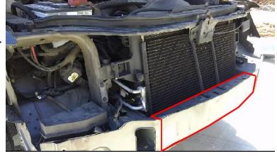
Update: If you have a sawzall, just cut right through both ends at the frame rails
