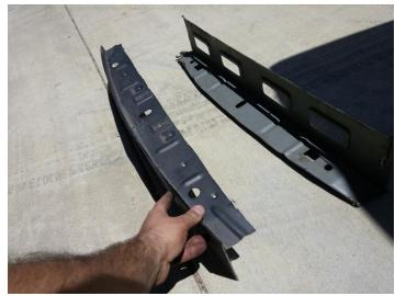
After you are finished cutting, this is how your Jeep should look on both sides of the chassis. These edges will be very sharp so don't touch with bare fingers. Now it's time to get the angle grinder with the grinding disk.
