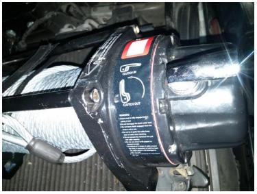
Unscrew all the bolts on the side of the winch where the clutch is located. No need to open the winch. Once the bolts are out, simply rotate the clutch forward. Reinstall the bolts and your good to go.
