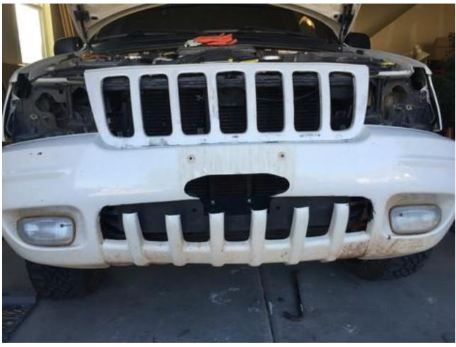
This is what your final install should look like. The lower plastic "7-slot" grill should rest under the winch mount.
