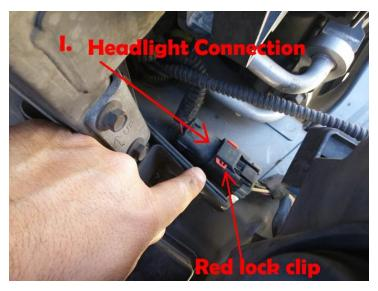
Once headlight support assembly is removed, this is what you should be left with...
