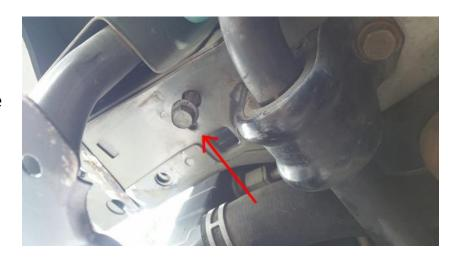
Step 2: Install the Hood Latch Support Brackets we have provided.
