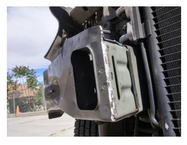
After you are finished cutting, this is how your Jeep should look on both sides of the chassis. These edges will be very sharp so don't touch with bare fingers. Now it's time to get the angle grinder with the grinding disk.
