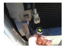
Step 8: H) Unscrew hood latch brackets with the T-30 Torx bit and remove both brackets. You will replace these by the longer brackets we have provided.
