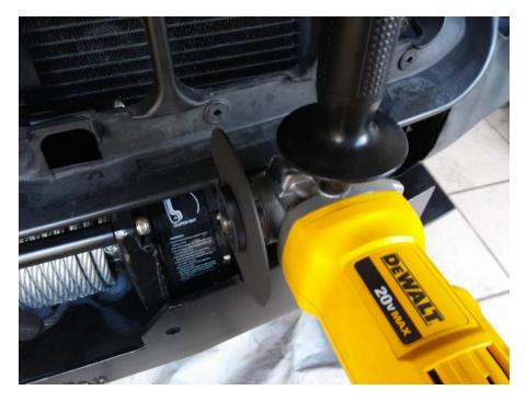
This image shows the winch installed with the clutch rotated forward and the small cut out in the headlight support.
