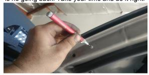
4e) Drll first hole with a 1/4" drill bit then enlarge hole with 23/64" drill bit.
