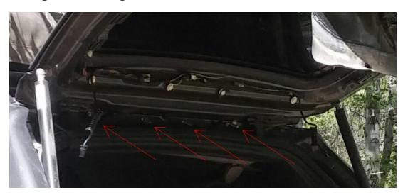
3E) Install the backing plates inside the hatch to the lower part of Kratos.
