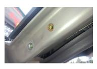
4h) With a 13mm socket, Install Reinforced Stud Mount using 8M-1.25 Bolt. Notice in the photo how the rivnut is perfectly aligned. Hand tighten 8M bolt until nice and snug. No need to use loctite as the bolt provided is a Serrated Flang-Nut bolt and it will not come undone on its own. If you would like to use loctite for added peace of mind, go right on ahead.
