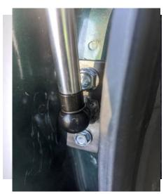
4k) Using 10mm socket and power drill, instal self tapping screws on the lower holes of the reinforced stud mounts.
