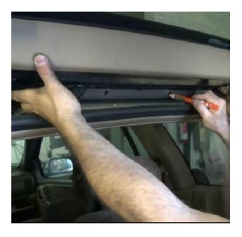
2c) Align plate and center the groove in the plate against the rubber seal on the hatch. With a pair of helping hands, hold plate in place and mark holes to be drilled.
