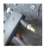
4g) Insert rivnut into the hole you just drill and with a strong steady grip, squeeze the rivnut until fully tight.
