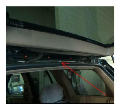
2d) Once the holes are marked, no need to remove the plate, just let it lay down as shown in photo. Drill marked holes to 1/2" drill bit. Start with a smaller bit as your pilot drill then drill to 1/2" OR USE STEP BIT
