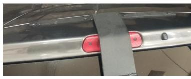
3C) Install the four bolts into carrier. Bolt size 3/8" x 1-1/4". Now SLOWLY open hatch making sure Kratos is sitting as flat as possible on the top of the hatch so it does not touch the roof while opening.
