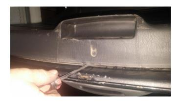
1c) Using a trim stick or equivalent, carefully pry the liftgate trim panel off the liftgate. There are 10 plastic fasteners used on the liftgate,
