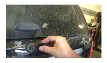
2a) Remove plastic cover on rear windshield wiper. Using a 13mm socket, remove bolt holding wiper into place and pull wiper off.
