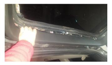
1d) Remove the black insulator cover from the liftgate. This is attached with a light adhesive and can slowly be pulled off.
