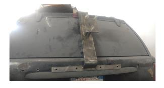
Mark four holes to be drilled and remove carrier from hatch.
