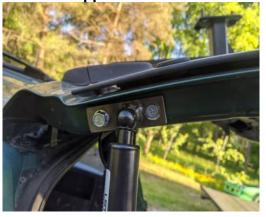
Remove pin on both ends of new strut and set aside.
