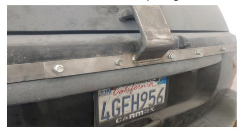
3D) With the hatch open, now it's time to wiggle that bar onto the four bolts. This part may be a PITA so take your time. Have some chamomile tea to keep your nerves calm and not go crazy and grow impatient. It will go on, just takes a little finesse. Use the 3/8" serrated flange nuts to tighten.
