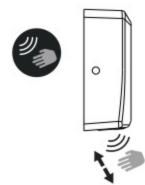
It is possible to adjust the sensor range by means of the sensor VR located on program PCB (See section 8 in "INSTALLATION").
