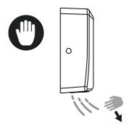
After 3 seconds without detecting hands, the device stops automatically.
