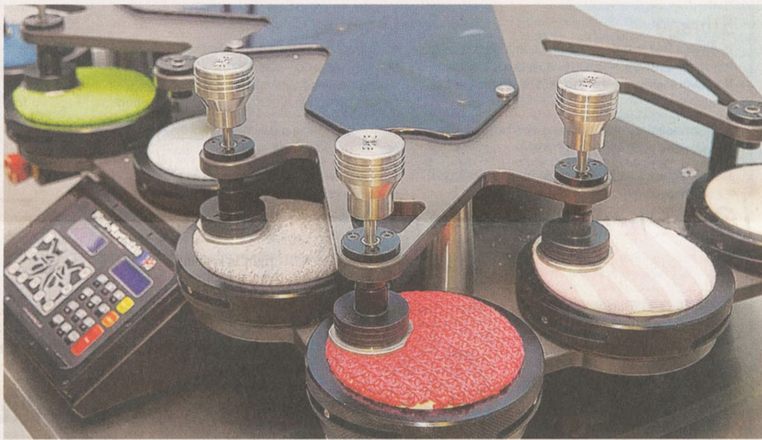
Sean Cormier, above, Fashion Institute of Technology assistant professor, puts sweater samples through the Martindale Pilling Tester, right. Below, he compares 'very severe' pilling on a blue, merino-wool swatch with a grading scale. Samples of cashmere (gray), cotton (light blue) and blends (green, striped) show varying degrees of pilling.
