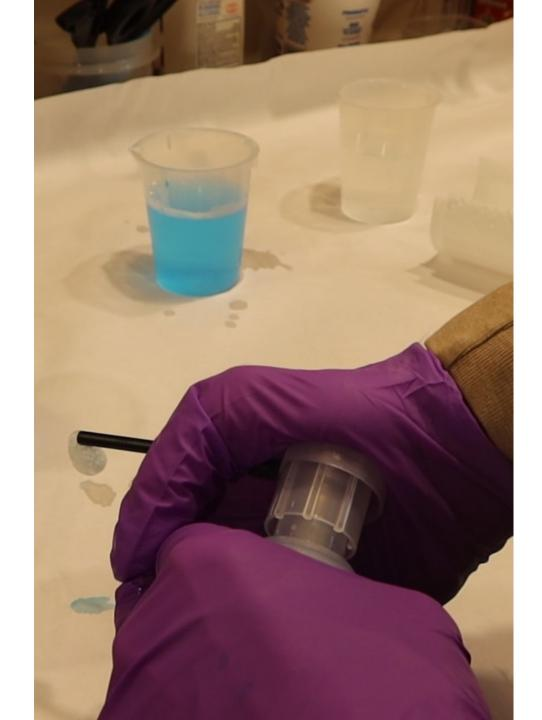
Gently press down on the actuator. You should hear a snap when it's in the correct position.
