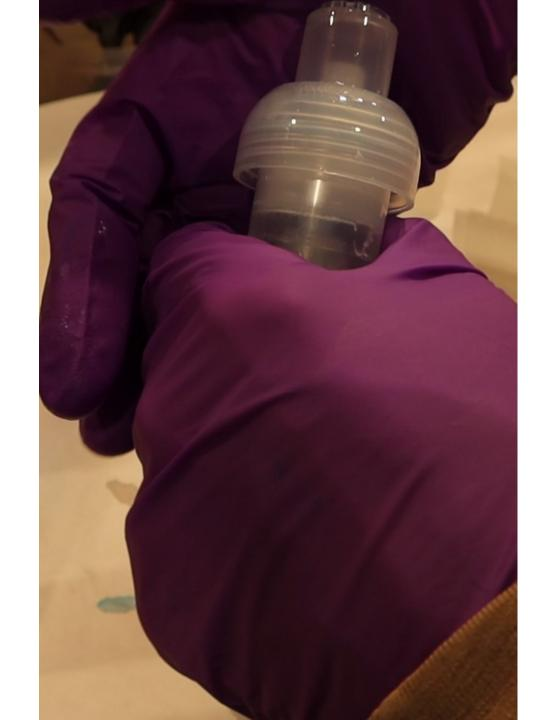
Press the threaded ring on. You should hear two snaps when it is in position. It should rotate but remain attached.
