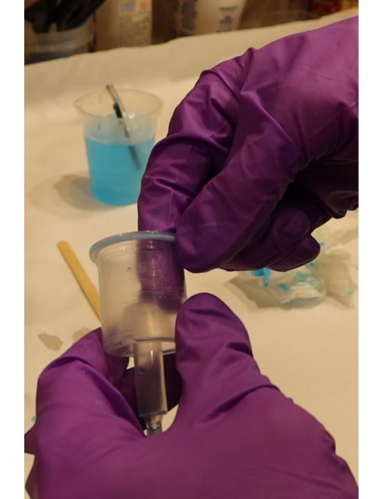
Spread silicone grease on the inside wall of the pump cylinder.
