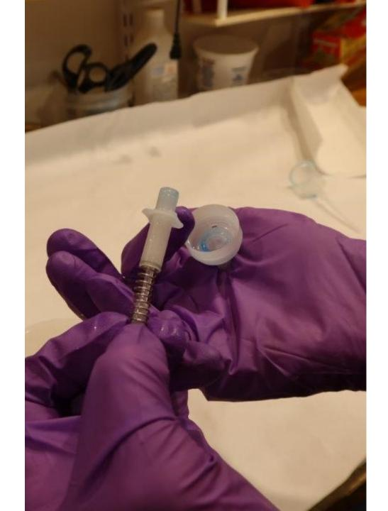
Remove the piston stem. Soak these parts in the soapy water.
