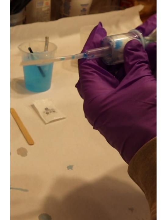
After soaking, clean out the pump cylinder with a paper towel.
