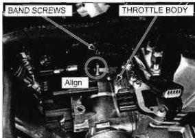
Tighten the insulator band screw so the insulator band distance is  $7.5 \pm 1$  mm (0.30  $\pm$  0.04 in).
