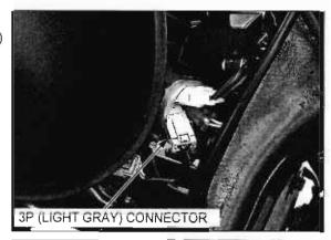
Check for continuity between the switch side connector terminals.
