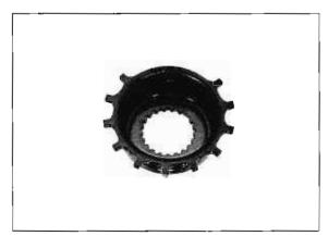
Check the primary drive gear for wear or damage.
