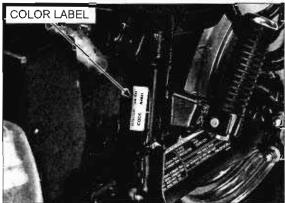
The Emission Control Information Label is attached on the left side of the frame down tube.
