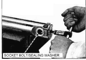
Do not remove the fork piston ring, unless it is necessary to replace with a new one.
