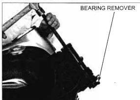
Install the steering stem nut onto the steering stem to prevent the threads from being damaged when removing the lower bearing inner race.
