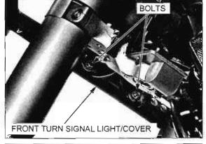
Remove the headlight unit (page 21-7). Disconnect the turn signal 3P connectors.
