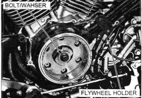
Remove the flywheel using a special tool.
