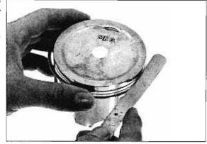
Insert the piston ring into the bottom of the cylinder squarely using the piston crown. Measure the piston ring end gap.
