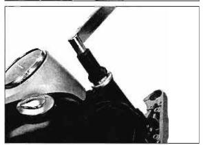
Install a new lock washer, aligning its bent tabs with the grooves in the steering top thread.
