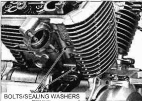
Remove the cam chain tensioner.
