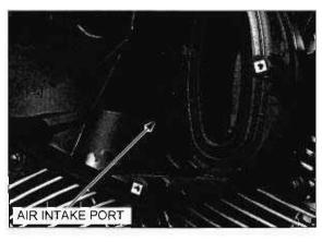
Start the engine and open the throttle slightly to be certain that air is sucked in through the air supply hose. If the air is not drawn in, check the air supply hoses for clogs and PAIR control solenoid valve (page 5-71).
