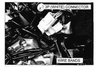
Release the wires from the clamps.
