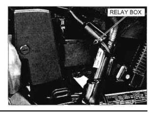
Release the tabs and remove the relay connector (Brown) from the connector cover.
