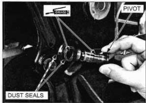
Install the middle rod joint with a new pivot bolt. Tighten the pivot bolt securely.
