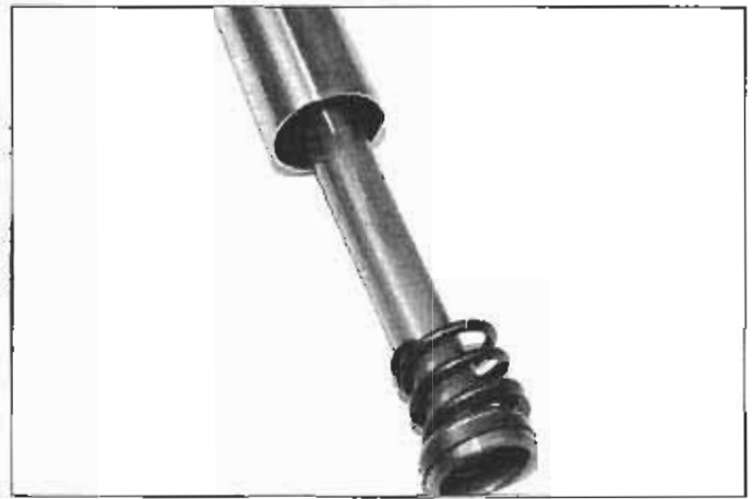
5.9b . . . and remove the damper rod and rebound spring from the other (upper) end of the fork tube
