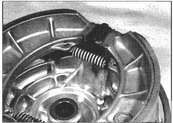
8.14a When installing the brake shoes, make sure the upper ends of the shoes are correctly seated against the brake cam ...
