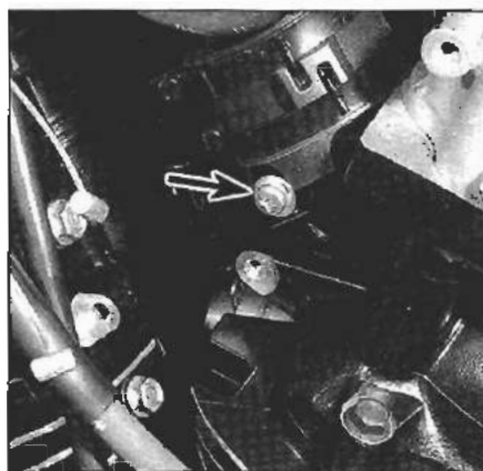
18.7 Remove the vacuum screw (arrow) from each intake port (rear cylinder port shown)
