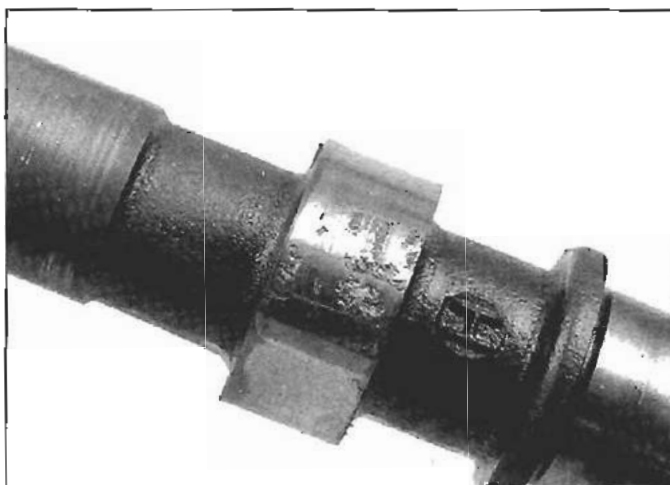
8.10a Inspect the camshaft lobes for wear; here's a good example of damage that will require replacement or repair of the camshaft
