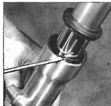
5.7 Pry the stopper ring out of its groove in the fork slider; don't distort this ring any more than necessary
