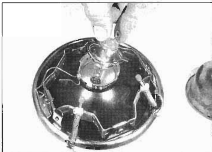
7.5 Lift out the bulb; don't touch the glass on the new bulb
