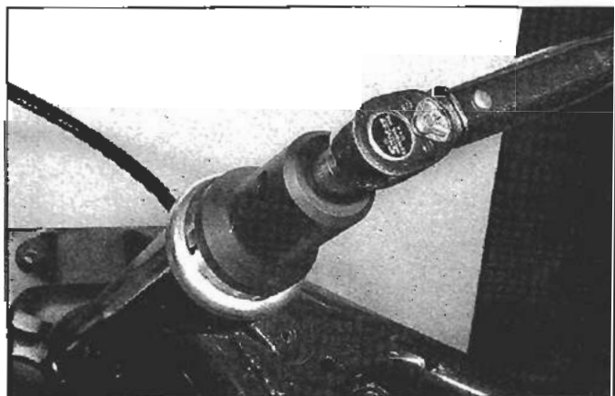
23.7 You'll need a special socket to torque the steering head bearing adjustment nut (it's available at Honda parts departments)
