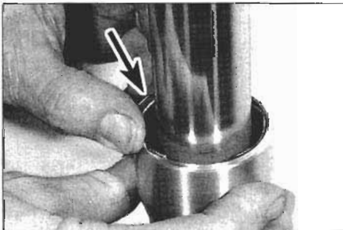
5.26 Compress the stopper ring and fit it securely into its groove in the fork slider (if the stopper doesn't "snap" into place, it's too fatigued to re-use)
