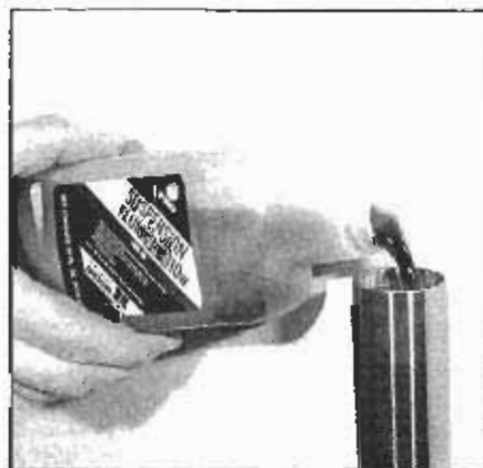
3.8 Add the specified type and amount of fork oil (fork removed from bike for clarity; it's not necessary to remove the forks to add new fork oil)
