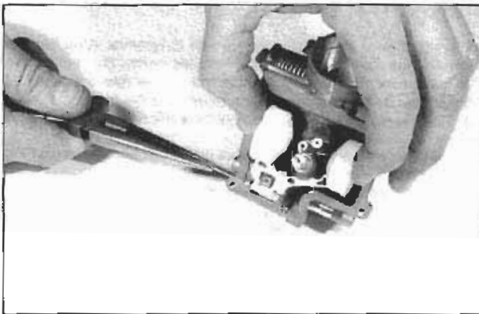
13.7 Pull out the float pivot pin and remove the float, needle valve and its retainer
