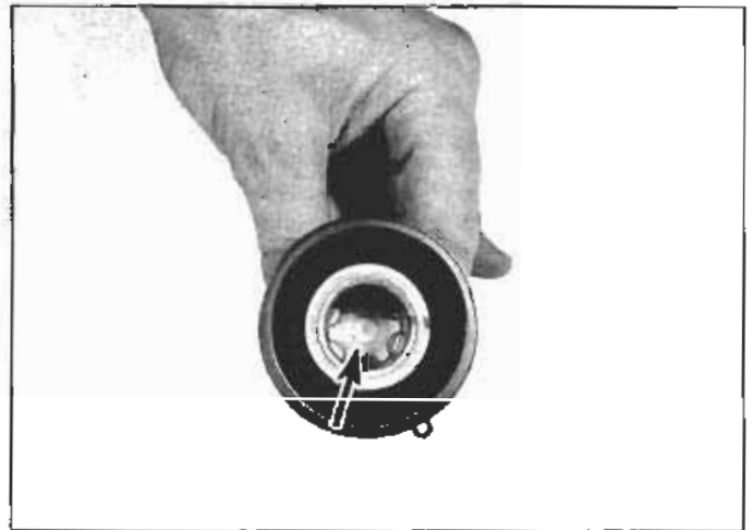
13.13 Push down on the jet needle holder with a Phillips screwdriver, turn it 1/4-turn counterclockwise, then remove the holder, spring and jet needle
