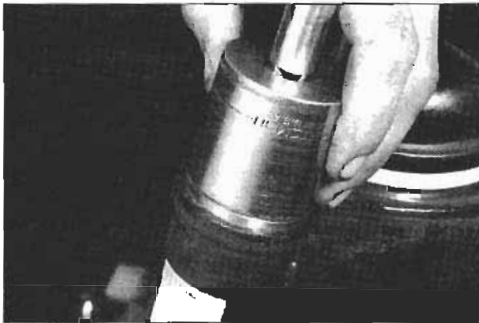
6.13c Tap the upper bearing outer race into position with the same tools
