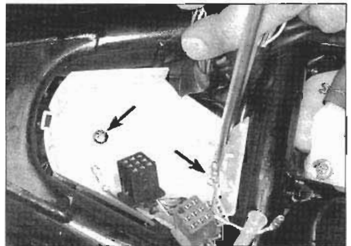
3.5b . . . label and disconnect the connectors inside the box, remove the box retaining screws (arrows) and remove the box
