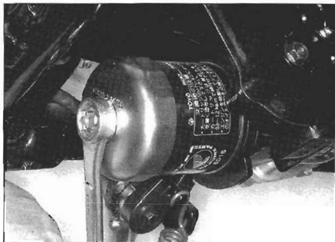
12.5b Use a filter wrench to remove the oil filter (if you don't have this type of filter wrench, use a pair of large water pump pliers)
