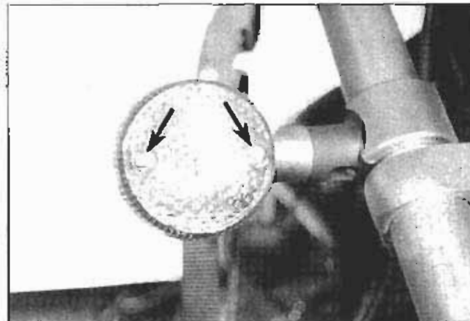
10.1 To detach a turn signal lens, remove these two retaining screws (arrows)
