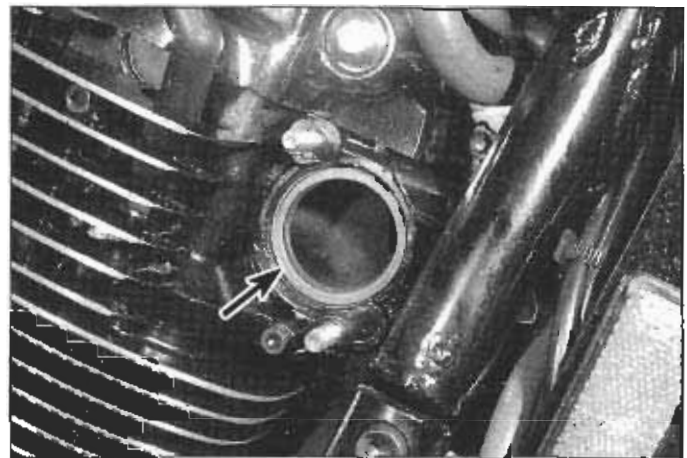
15.1c After detaching the exhaust pipes from the heads, carefully pry out the old gaskets (arrow)
