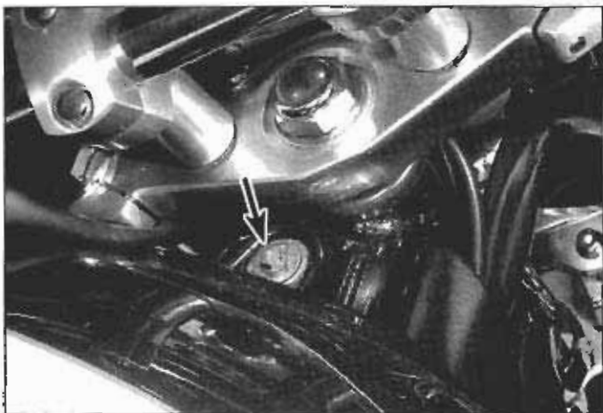
2.25 Remove the front fuel tank mounting bolt (arrow) and collar; replace the rubber insulator if it's damaged
