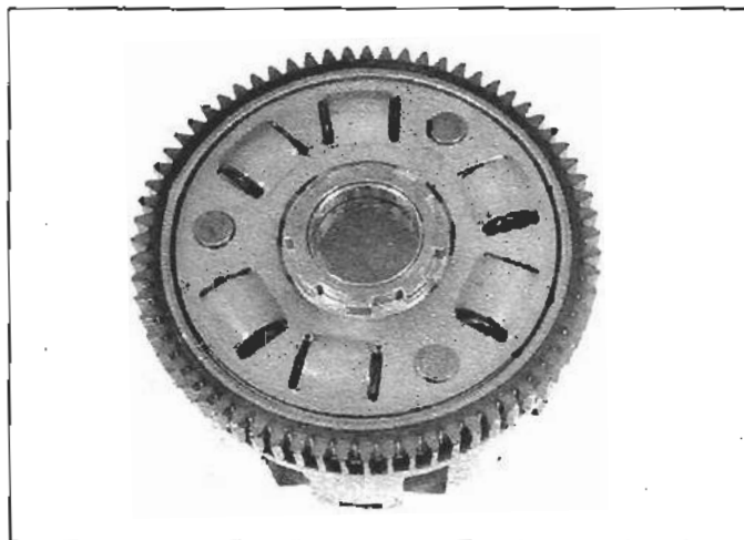
18.62 Inspect the primary driven gear teeth on the backside of the clutch housing; if the teeth are worn or damaged, replace the clutch housing
