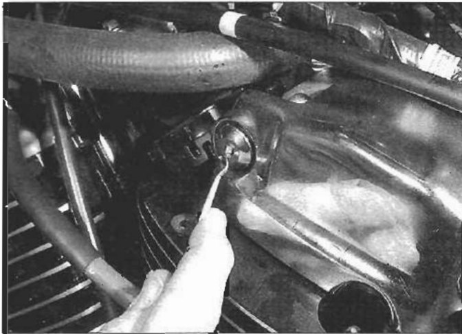
5.10a Before removing the engine from a VT1100C2, VT1100T or a 1997-on VT1100C model, remove all four cylinder head cover shrouds: first, pry out the small plugs from each Allen bolt . . .
