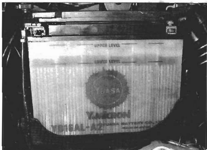
4.4 The electrolyte level should be between the marks on the battery case
