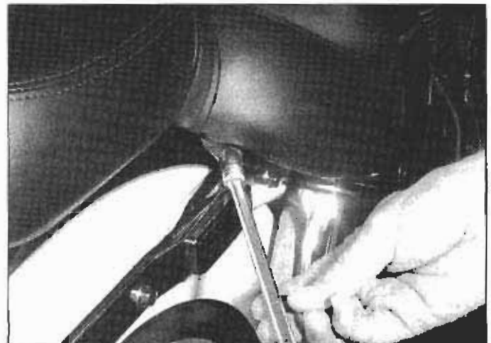
6.3b . . . and remove the two side bolts (one on each side)
