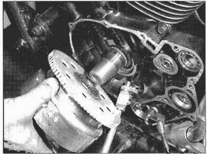
32.12 With the needle bearing and Woodruff key in place, install the assembled flywheel/starter driven gear onto the crankshaft
