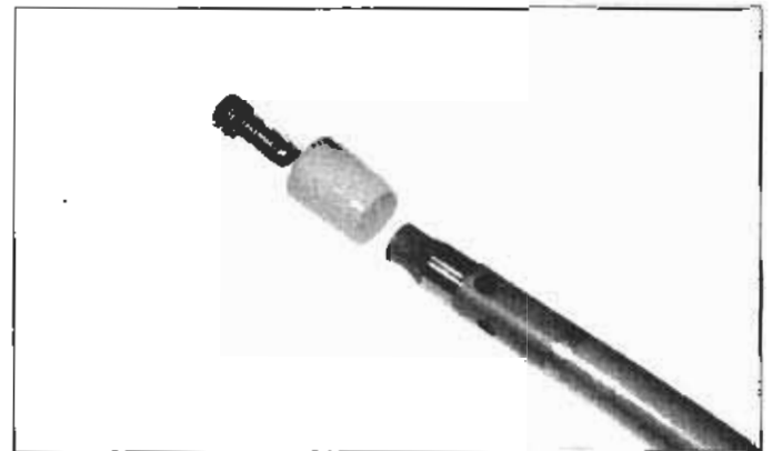
5.22 The damper rod bolt, lock piece and damper rod fit together like this in the lower end of the slider (slider not shown)
