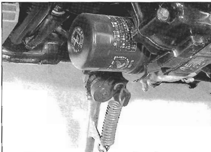
12.5a The oil filter (arrow) is at the left lower rear of the engine; the easiest way to reach it is from the right side, with the bike leaned over to the left on its sidestand
