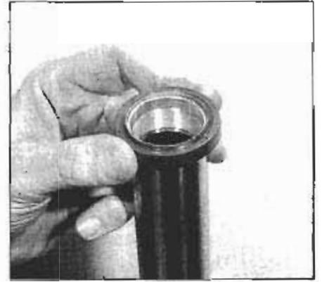
5.25b . . . and install the seal on the fork tube; don't let the upper edge of the fork tube damage the seal lip
