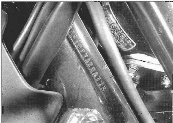
The frame serial number is stamped into the right side of the steering head
