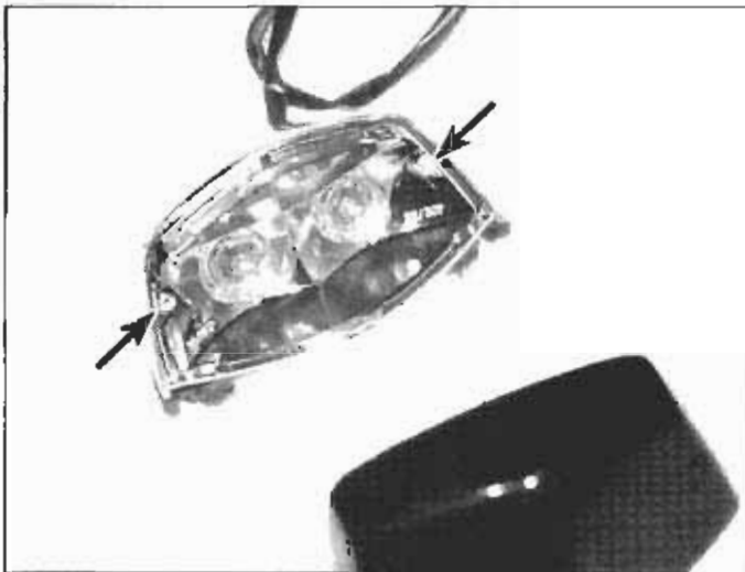
10.5 Remove the brake light lens screws (arrows) and take off the lens
