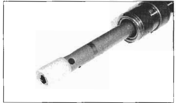
5.20 Install the lock piece on the lower end of the damper rod
