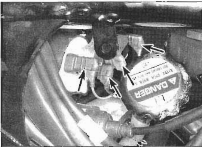
3.3a The primary terminals (arrows) for both coils are on the front ends of the coils
