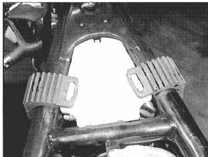
13.2 To remove the connector box cover, disengage these two rubber straps from the cover tabs
