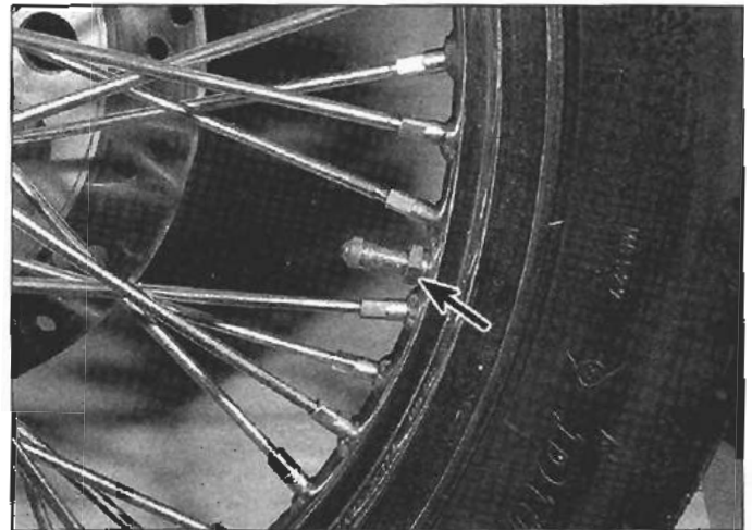
8.5 Make sure the tire valve locknut (arrow) is snug and the valve cap is tight
