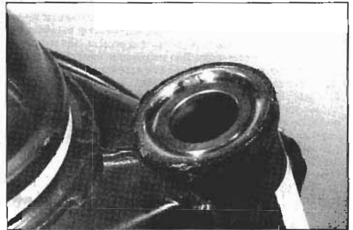
6.13d . . . the upper bearing outer race should look like this when installed
