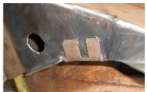
Bend the tab upward. Slot in tab needs to be as low as possible. Once folded, cut out the top of tab.
