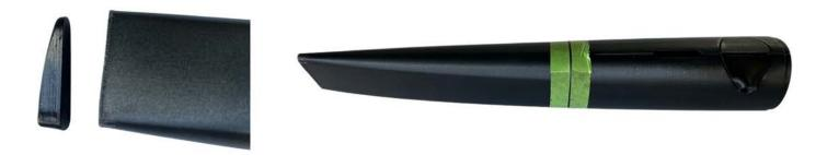
Apply a thick layer of adhesive (read adhesive manufacturer's instructions) to the for'd section of the pre bonded parts 3 & 4 then slide the bow section 2 over sections 3 & 4 ensuring that the centre line is matched up.
