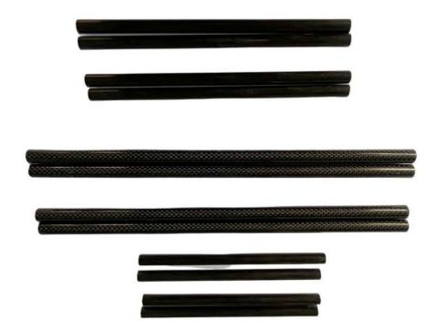
Note that the 95 mm end of the beam fits into the DF hull deck beam support and the 75 mm end slides into the pre bonded tube on the Amas all 4 beams are the same length.
