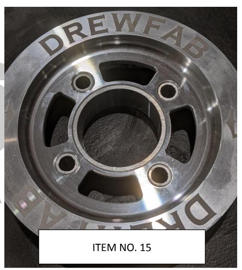
• Install the pulley with 3/8-16 x 1-3/4 allen head bolt and washers.
