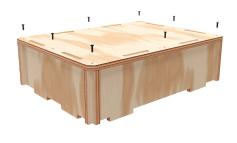
INTERLEAF CRATES ARE DESIGNED SO THAT THE TOP END PANEL FITS ONE SIDE OF THE VERTICAL TABS PROTRUDING FROM THE SIDE PANELS AND THE BOTTOM END PANEL FITS THE OTHER SIDE UNIQUELY.
