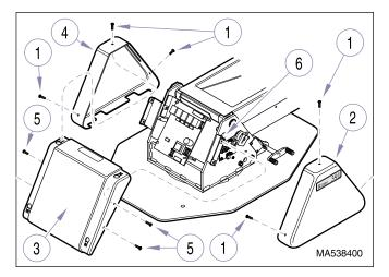
Figure 4-12. Covers Removal / Installation
