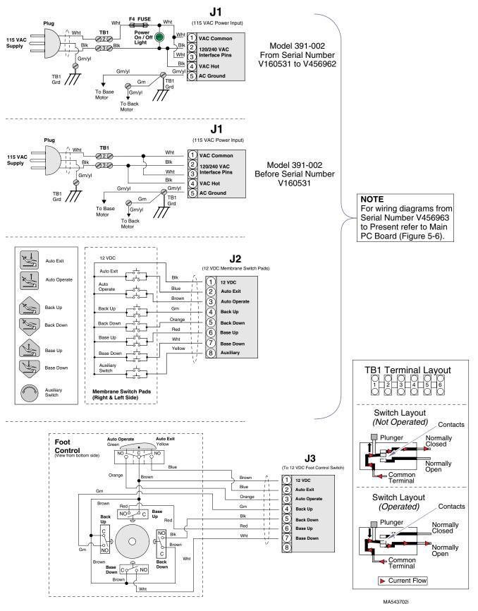
Figure 5-3. Main P.C. Board Plug Connectors (J1, J2, J3)
