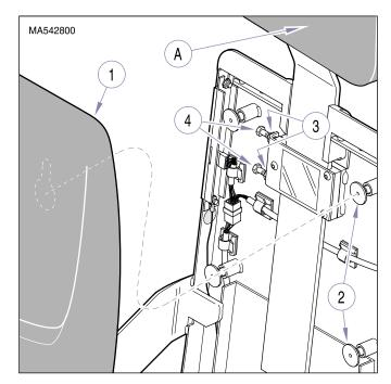
Figure 4-27. Headrest Slide Adjustment
