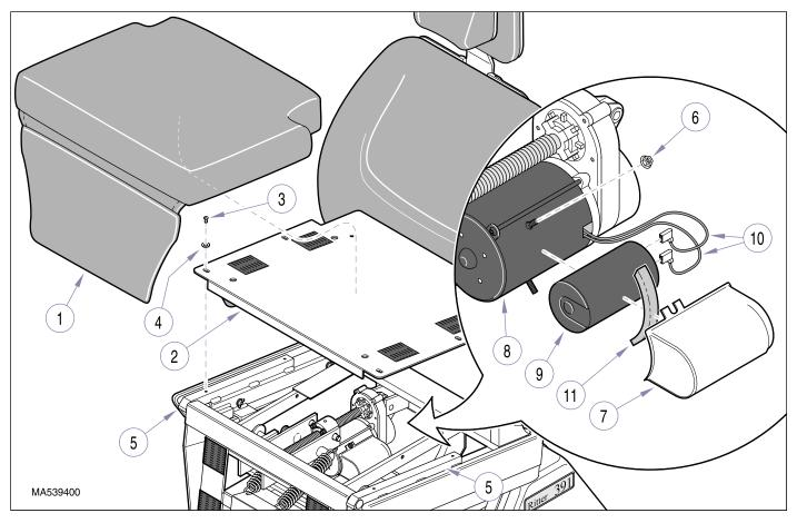
Figure 4-9. Back Capacitor Removal / Installation
