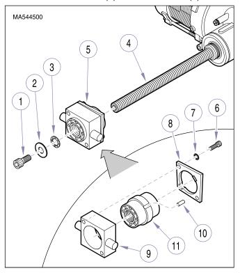
Figure 4-32. Base Motor Trunnion / Drive Nut Removal / Installation
