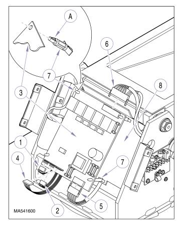
Figure 4-13. PC Circuit Board Removal / Installation
