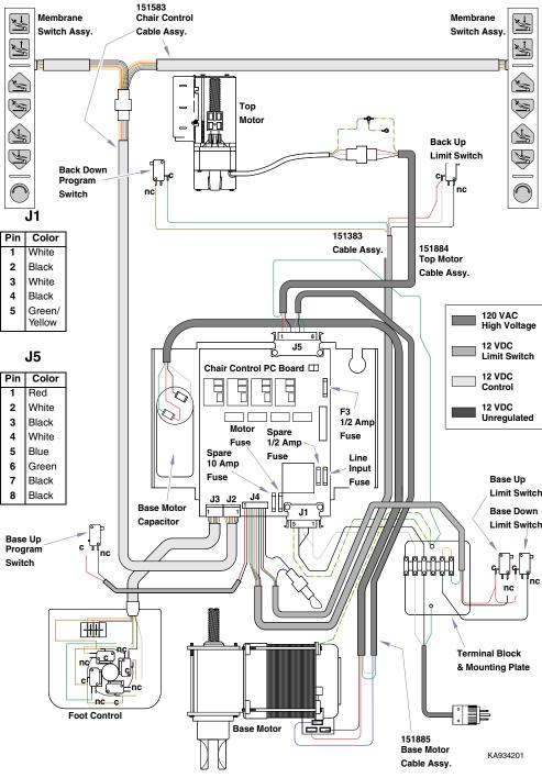
Figure 5-1. Wiring Diagram (120 VAC Units) Thru Serial Numbers V160530
