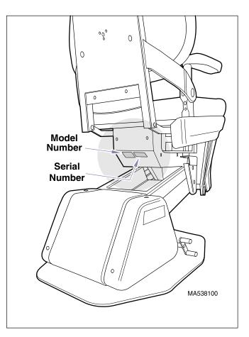
Figure 1-3. Model Number / Serial Number Location
