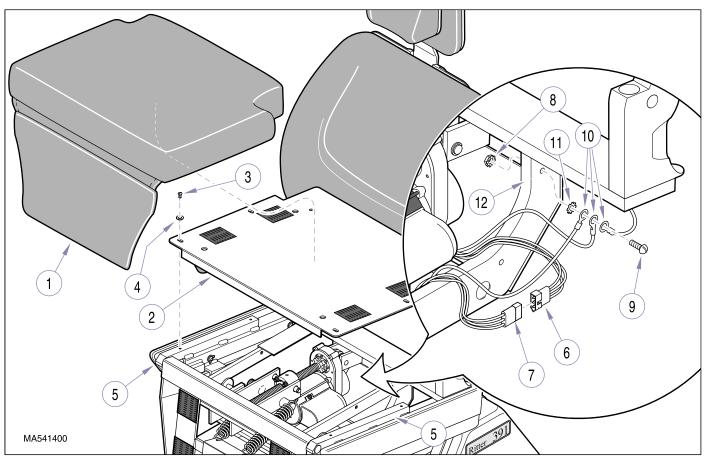
Figure 4-10. Back Motor Wire Harness Disconnection / Connection
