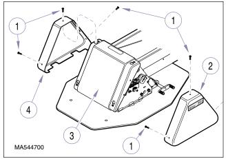
Figure 4-25. Covers Removal / Installation
