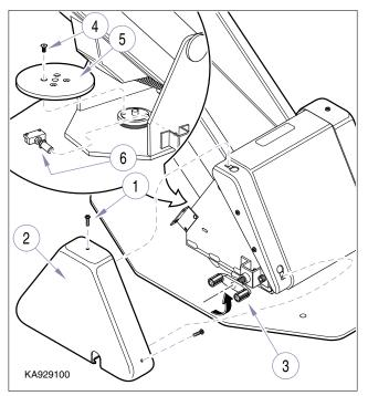
Figure 4-22. Lock Block Removal.
