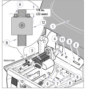
Figure 4-11. Back Motor Removal / Installation
