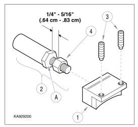
Figure 4-23. Lock Block Disassembly.
