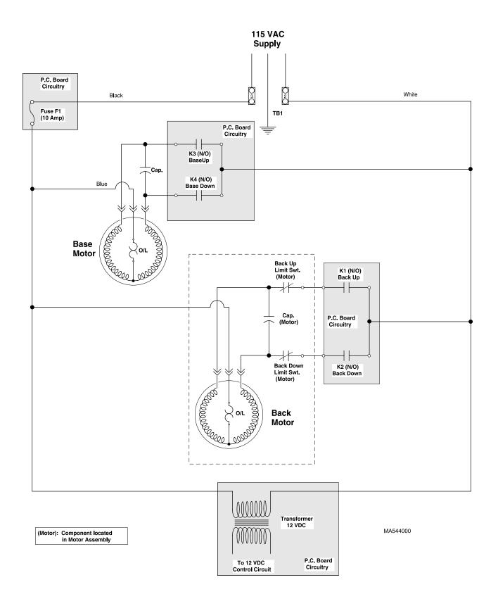
Figure 5-8. 115 VAC Motor Circuit
