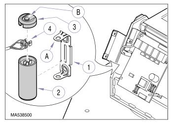
Figure 4-2. Base Capacitor Removal / Installation
