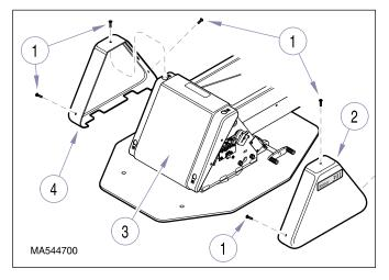
Figure 4-30. Covers Removal / Installation
