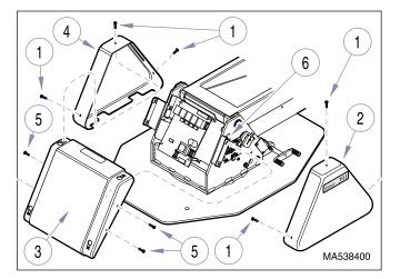
Figure 4-22. Covers Removal / Installation
