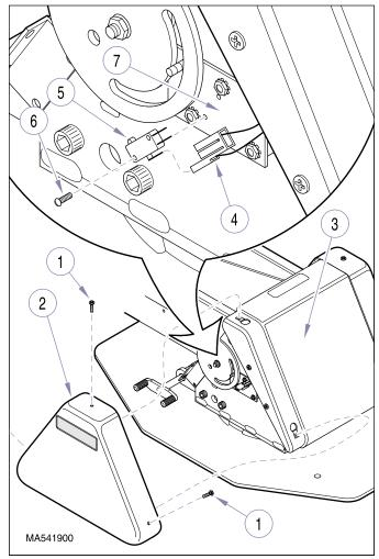
Figure 4-16. Base Up Program Limit Switch Removal / Installation
