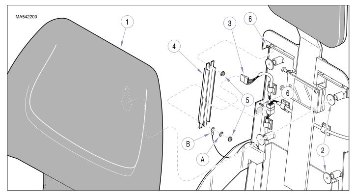
Figure 4-19. Membrane Switch Panel Removal / Installation
