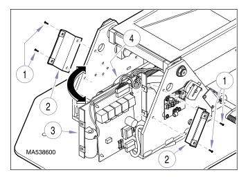
Figure 4-4. Base Motor Access
