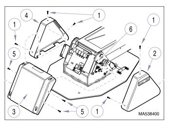
Figure 4-1. Covers Removal / Installation
