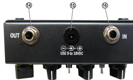
**IN Jack (#16 on above diagrams):** Connect a shielded (1/4" mono plugs) cable from your instrument into this jack. Always use good quality shielded cables (e.g. Fulltone Gold Standards) for audio signals, speaker cables are un-shielded and should not ever be used to connect your instrument to other effects or your amp.
