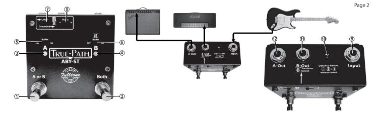
Input: (see #9 on above diagrams) Connect a cable (shielded with 1/4" mono plugs) coming from your guitar, bass, or other instrument into this jack. Always use good quality *shielded* cables (eg.Fulltone Gold Standards) for audio signals, speaker cables are *un-shielded* and should not ever be used to connect your instrument.
