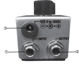
**IN Jack** (#1 on above diagrams): Plug a cable (shielded with 1/4" mono plugs) coming from the instrument (or from the OUT of other effects) into this jack. Always use good quality shielded cables (e.g. Fulltone Gold Standards) for audio signals, speaker cables are un-shielded and should never be used.
