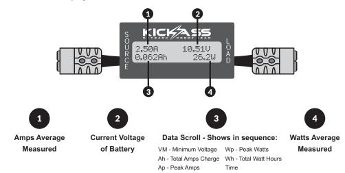
Data Scroll - When power is supplied to the watt meter the unit will start recording data. To reset the Data Scroll to zero simply disconnect the watt meter from power, wait 30 seconds and reconnect.
