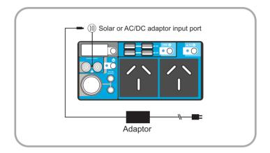
Plug the AC/DC Adaptor provided into both the wall and the DC charging port on the unit. The LCD display will flash to confirm the charging process is underway. When the battery is fully charged, the LCD will display "FULL" and the Charging LED indicator will be green.
