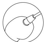
The cable will magnetically attach into place. The power button LED will pulsate slowly to indicate charging.
