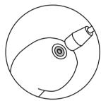
The charging contact is a small metal circle located on the bottom of the device. Line up the charging cable with the contact.
