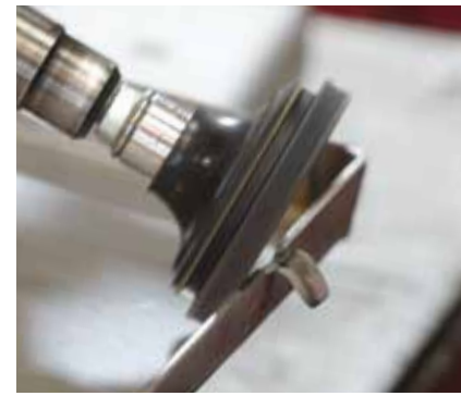
Edge chamfering a fabricated stainless component.
