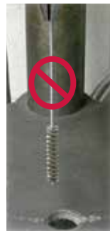
Incorrect Mounting in Chuck
