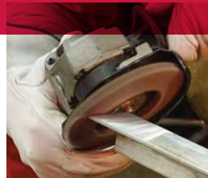
Chamfering an aluminum extrusion preparing for weld
