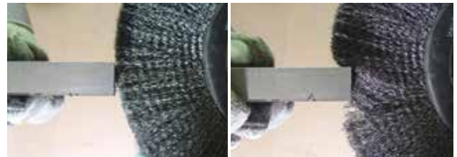
Correct Wire Tips Doing the Work
