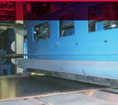
Removing light corrosion and mill scale from coiled steel.
