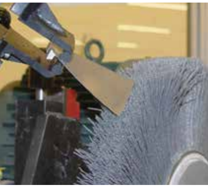
Deburring the tip of a turbine blade.
