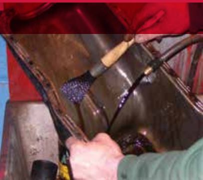
Cleaning an oil pan with a parts cleaning brush.
