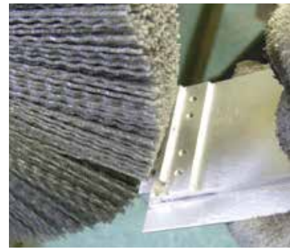
Removing burrs from an aluminum heat sink.
