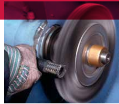
Removing rubber coating from a hydraulic hose.
