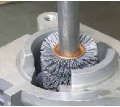
Deburring internal bores of a cylinder head.
