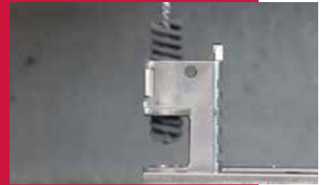
Deburring cross holes in a firearms component.
