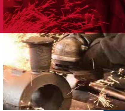
Riser removal with a type 27 grinding wheel.
