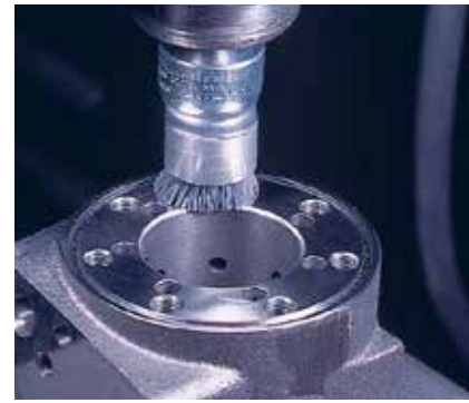
Blending tool marks on a hydraulic component.
