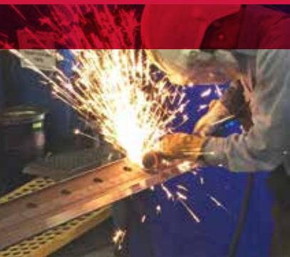
Using a cone to clean surface imperfections.
