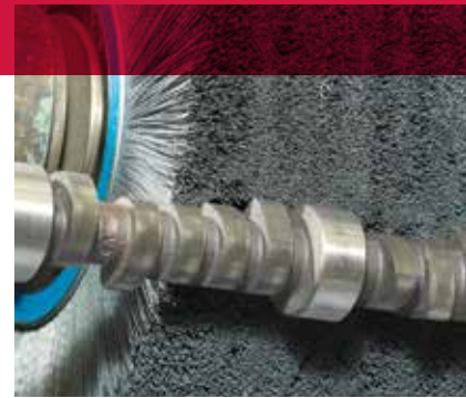
Deburring a camshaft with a Nylox wheel.
