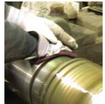
Polishing a rail axle journal with a non-woven hand pad.
