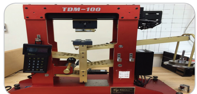
The TDM100 test machine measures cut resistance of glove fabric to a sliding blade.
