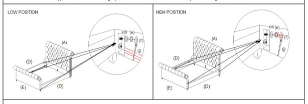
Step 6. Install the Side rail (D) into Headboard (A) then Footboard (E) with Nut (f), Bent washer (e) and Flat washer (d), use Wrench (j) to tighten the nut.
