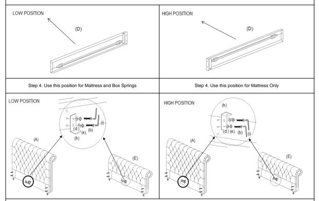
Step 5. Install the Angle iron (h) to the headboard (A) and footboard (E) with Inner hexagon screw (b), Bent washer (e), Flat washer (d) by Allen wrench (i), make sure it is in the right position and direction as shown in the picture and tighten the screws.
