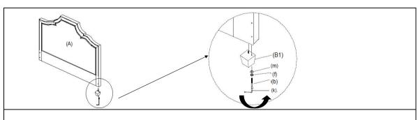
Step 1. Install the Headboard foot (B1) to the Headboard (A) with Flat washer (m), Bent washer (f), Allen head boit (b) by Allen Wrench (k).
