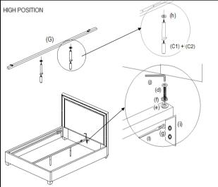
Step 7. Screw in the Middle leg II (C2) into Middle leg rail (G) with plastic washer (h), then install the Middle leg rail into Angle iron (i) with Inner hexgon screw (d), Bent washer (f), Flat washer (e) by Allen wrench (j),then, use the Wrench (l) to tighten the Nut (g) and Innger hexgon screw (d). There is an adjuster under the Middle leg, you may need to adjust it a little bit to touch the floor.
