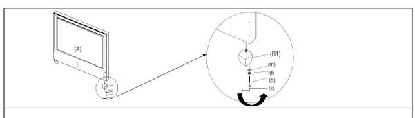
Step 1. Install the Headboard foot (B1) to the Headboard (A) with Flat washer (m), Bent washer (f), Allen head bolt (b) by Allen Wrench (k).
