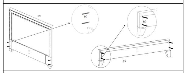
Step 3. Screw in the Threaded bolt (a) to the Headboard (A) and Footboard (E), and tighten the threaded bolts by hand.
