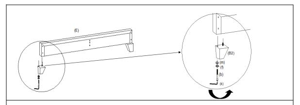
Step 2. Install the Footboard foot (B2) to the Footboard (E) with Flat Washer (m), Bent washer (f), Allen head bolt (b) by Allen Wrench (k).
