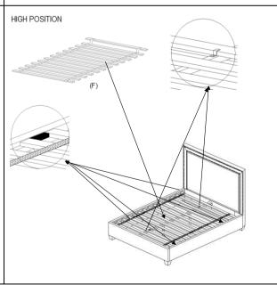
Step 8. Put the SLAT (F) on the rails , lock it as shown and make it parallel.
