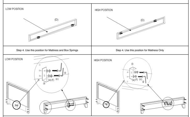
Step 5. Install the Angle iron (i) to the headboard and footboard with Inner hexagon screw (c), Bent washer (f), Flat washer (e) by Allen wrench (j), make sure it is in the right position and direction as shown in the picture and tighten the screws.
