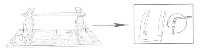
Then fix the Both legs with table top tighten the bolt on respetive holes showen on diagram.
