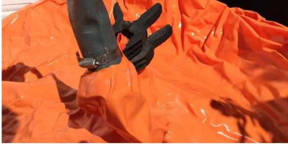
3. Once filling is complete roll up top and use the attached tie to secure filler tube, ensuring that it is closed.
