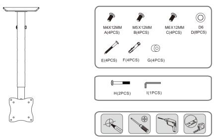
STEP1 Attach the frame to the post
