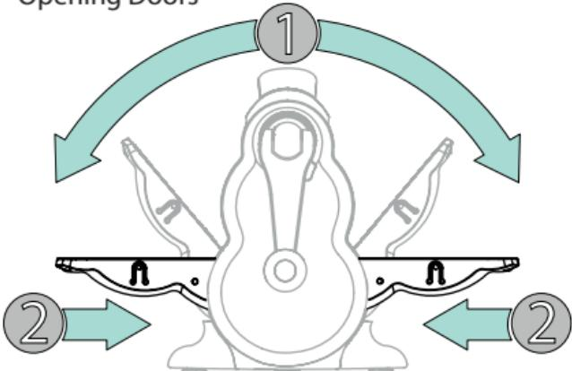
To open the machine, (1) pull down the beds from the centre using the finger grooves as a guide. (2) Once horizontal, push both beds in toward the centre of the machine to lock in place. To fold away, pull beds away from the centre using the finger grooves on the beds for grip. Once unlocked, fold beds up.
