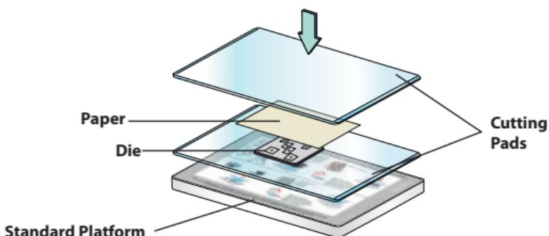
1. Place Sizzlits die onto a Cutting Pad with foam side up. Place paper over the die. Place another Cutting Pad over the paper to create a "sandwich."
