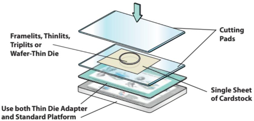
1. Place material to be die-cut on Cutting Pad. Place die over paper or photo and align. Place another Cutting Pad over the die and paper to create a "sandwich."
