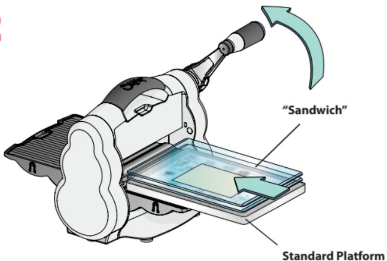
2. Place "sandwich" on the Standard Platform and slide Platform into opening of Big Shot Foldaway. Note the rotation of the handle and continue to rotate it in the same direction until the Platform has passed through the opening and the rollers. Remove Platform from Big Shot Foldaway. Your die-cut shape is ready to use!
