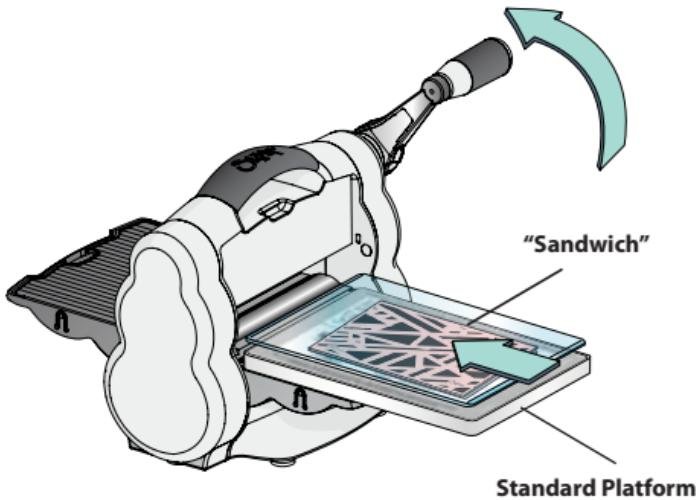
3. Place "sandwich" on Standard Platform and slide Platform into opening of Big Shot Foldaway. Note the rotation of the handle and continue to rotate it in the same direction until the Platform has passed through the opening and the rollers. Remove Platform from Big Shot Foldaway. Your embossed material is ready to use!
