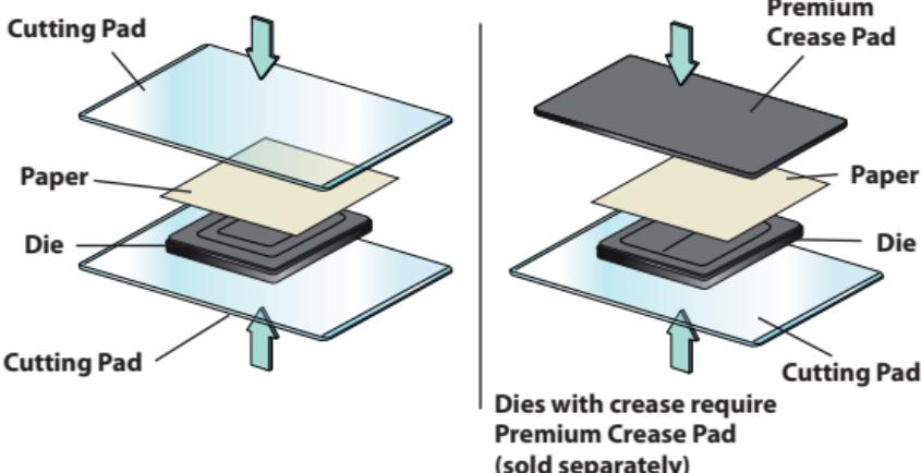
1. Place an Originals or Bigz die on a Cutting Pad with foam side up. Place paper or desired material to be cut on top of the die. Place the second Cutting Pad or Premium Crease Pad on top of the paper or material to create a "sandwich."
