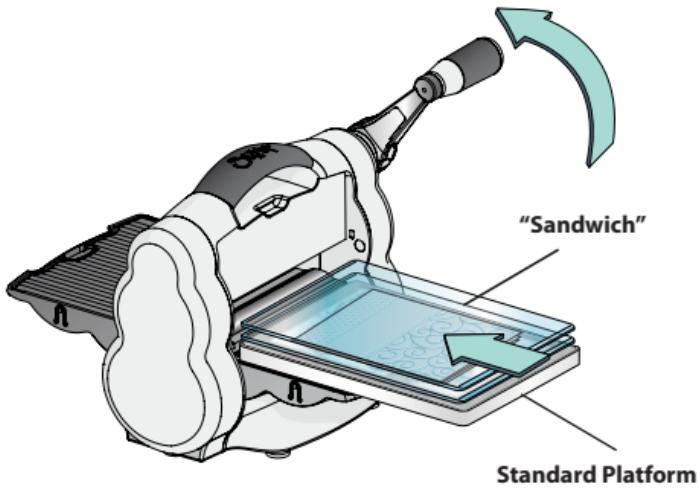
Place "sandwich" on Standard Platform and slide Platform into opening of Big Shot Foldaway. Note the rotation of the handle and continue to rotate it in the same direction until the Platform has passed through the opening and the rollers. Remove Platform from Big Shot Foldaway. Your embossed material is ready to use!
