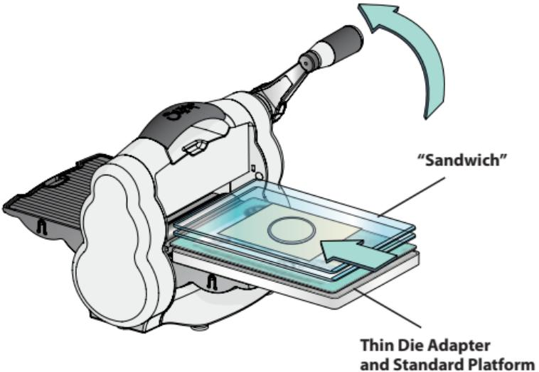
2. Place "sandwich" on both Thin Die Adapter and Standard Platform and slide platform into opening of Big Shot Foldaway. Note the rotation of the handle and continue to rotate it in the same direction until the Platform has passed through the opening and the rollers. Remove Platform from Big Shot Foldaway. Your die-cut shape is ready to use!
