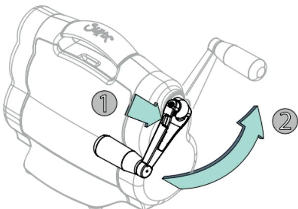
To begin using the machine, (1) press the lever in on the crank shaft to release the handle. (2) Lift the handle up vertically and pull it down so that it is parallel with the machine. The crank shaft will lock in place once it is in position. To store away, press the lever to release the handle from the locked positon and twist up and down in front of the machine to lock in place.
