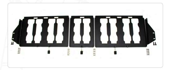
Line up all bolt holes with each plate. Assemble the plates using 8 of the M8 bolts and lock nuts. Insert each bolt and hand thread all nuts onto each.
