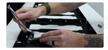
Keep the plate assembly upside-down to install the end mounts. Each end mount is different. There's a driver-side and passenger-side version. When mocking them up, the larger angle should be facing the top of the plates.
