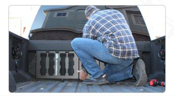
Hand thread each T40 mount bolt into the factory, threaded holes. Snugeach bolt sufficiently using either a ratchet or an impact. **Do not overtighten.**
