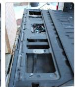
Locate and remove all 8 screw retainers from the tailgate using a standard screwdriver.
