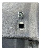
Note: if your tailgate has been bed-lined, first cut away the bed-liner from the screw retainers using a razor blade.
