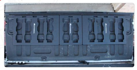
Insert the T25 bolts through the mount holes in each plate according to the diagram below.
