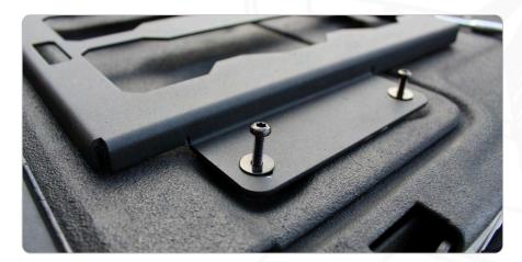
Using the  $\frac{1}{4}$ " ratchet and T25 Torx Socket, tighten all 8 bolts. Do not over tighten. Pull up on each plate to ensure all well nuts are fully seated.
