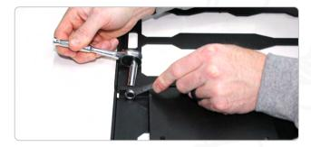
Using the T25 Torx Bit (Some models have T20 screws), remove all 8 screws and the tailgate access panel.
