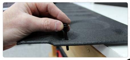
If your truck has a spray-on bed liner, the bolts may not easily fit through some of the holes. These holes need to be opened up with a drill and 1/4" bit.
