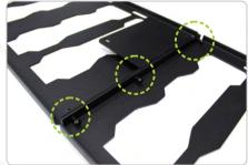
Using the ratchet, 8mm socket, and 8mm wrench tighten all 6 nuts. Ensure all are snug but do not overtighten.
