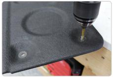
Reinstall the tailgate access panel. Line up all 8 holes with the hole in each well nut. Place the 8 spacers over each bolt hole.
