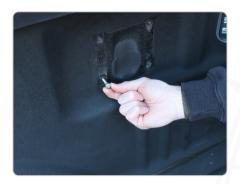
**d.** Finish threading the bolt using either the hand ratchet or an impact driver.
