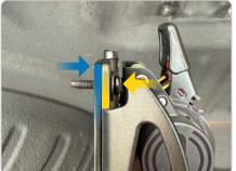
Hand thread each bolt into the Boxlink mount. Repeat for the other side. Add and hand thread the bottom two bolts.
