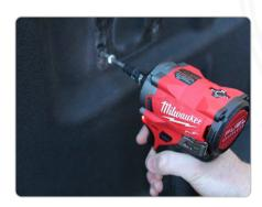
c. Using the T30 torx bit and bit driver (or ratchet), thread the bolt about 25% of the way into the hole.
