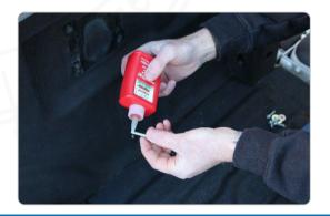
**b.** Begin threading the bolt into one of the 4, predrilled boxlink bolt holes by hand.
