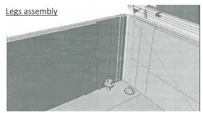
Insert the pin of the leg inside the holes
