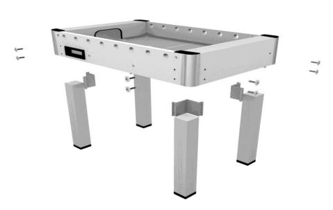
Set the L shaped bracket internally the table body and insert the aluminium leg inside the L bracket. To block them, insert from the external of the body the screws 8x45 with washers 8x32 and tighten them up with the allen screw.
