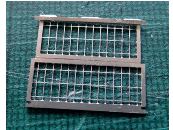
Fig 3: Having folded and glued the door locking bar in place, the remaining etched fold is visible.
