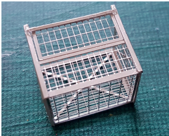
Fig 7: The completed etched cage.
