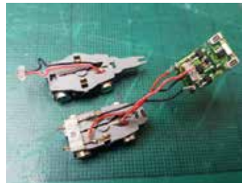
Fig 13: The modified KATO chassis at the bottom, with an unmodified example for comparison.
