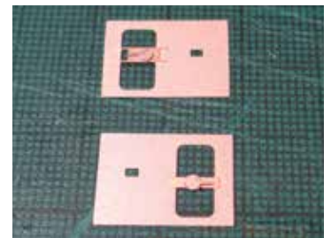
Fig 8: Laminated AK6 specific side panels.
