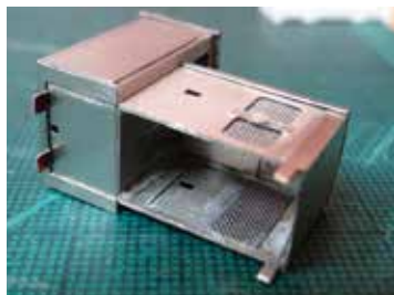
Fig 10: The mesh fitted and the locating tabs bent downwards.
