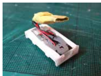
Fig 15: The completed KATO chassis. We recommend black tape to stop the board showing through the side grilles.
