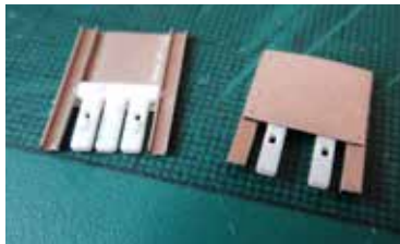
Fig 16: Assembled armour plates (rear on the left, front on the right).
