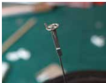
Fig 9: Completed brake wheel prior to fitting.
