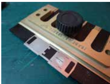
Fig 4: Using a Hold-and-Fold to fold two of the door edges in one go.
