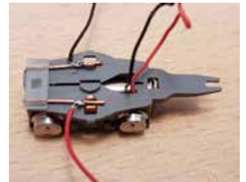
Fig 14: A close up of the 3D printed clip holding the phosphor bronze rods in place against the pickups.
