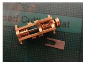
Figure 1: Chassis with layshaft fitted.
