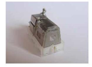
Figure 5: The completed body prior to painting
