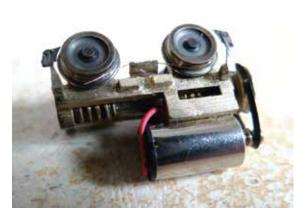
Figure 4: Completed chassis showing pickups and brake shoes
