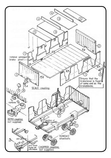
(6) in relation to the larger axleboxes (brake end). Fit brake blocks last.
