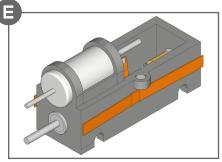
Push motor gently into the mounting with the power tabs towards the centre of the chassis. Slide this gently as it is a tight fit. NOTE: the '+' pin has an indented circle in the assembly drawing, the tabs should be orientated as per the diagram. Gently move the phosphor bronze pick up tabs so they push on to the power tabs on the motor. NOTE: No glue or solder is required.
