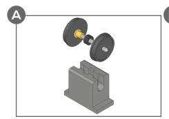
Remove one wheel from the axle. Thread one bush and slide on the plastic gear to the axle. Sliding the gear into the slot in the gauge, push the gear into the centre of the axle by pressing firmly on the wheel. Fit the second bush, and then press the other wheel firmly in place. Repeat for the second axle.
