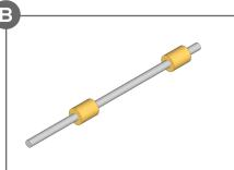
Fit the two brass worms to the layshaft, position is approximate as per template below. Use tapered reamer to ensure these are a tight fit. Secure with Loctite 603 'thread lock'. NOTE: this is not superglue, but a retaining compound.
