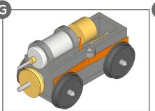
Apply a very small amount of lubricating oil to the roller bearings on the layshaft, the worm gears on the layshaft and the wheel axles where they pass through the bushes.
