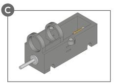
Apply a small drop of Loctite 603 to the non-drive end of the layshaft (this will have a shorter length of shaft beyond the brass worm). Push firmly into the roller bearing in the chassis so the tip is flush and wipe off any excess Loctite immediately. After ten minutes, place the chassis on a firm surface with the layshaft pointing upwards. Thread a second roller bearing onto the layshaft and push this firmly into the chassis being careful not to dis-lodge the existing bearing.
