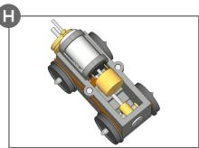
Fit the belt to the pulleys, being careful this is not contaminated with oil, and test run the chassis. It will require gentle running in to improve it's performance. We recommend 15 minutes at half speed in both directions.
