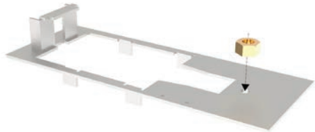
Figure 9– Front chassis support and carrier 10BA nuts
