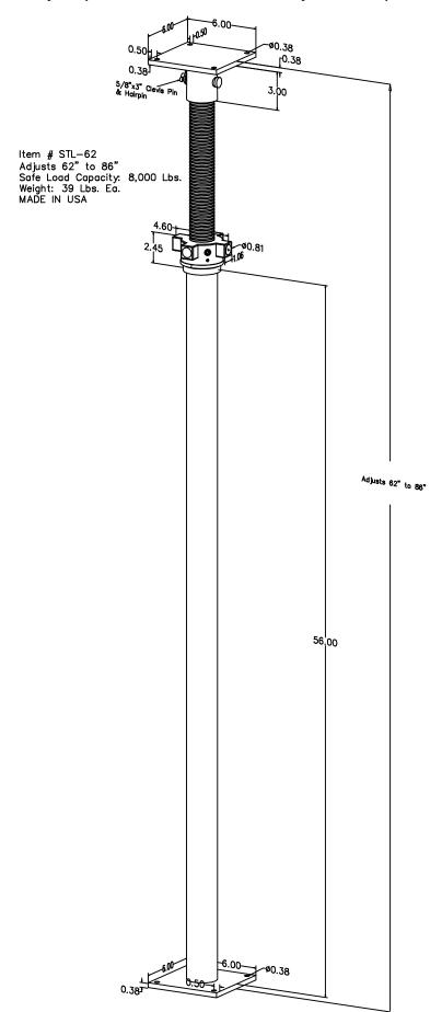
Use Turning Bar as lever for height adjustment (Item # MJ-TB12, MJ-TB24, MJ-TB36).
